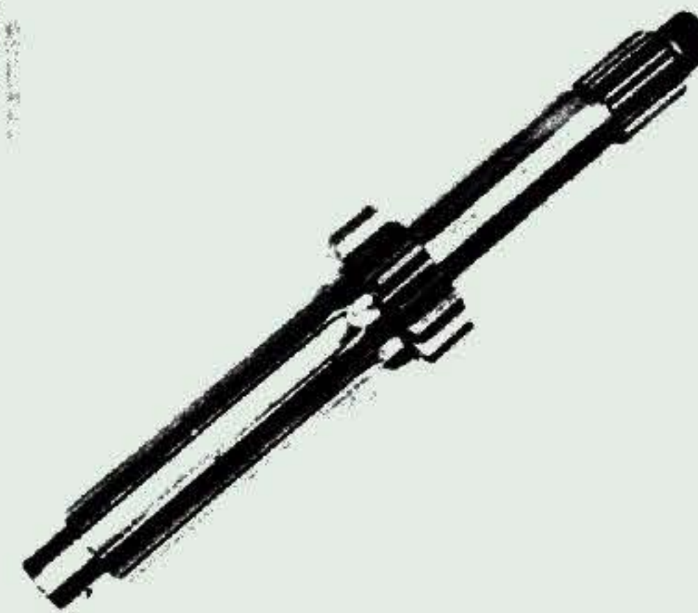
35.1a The gearbox mainshaft and 1st gear pinion
