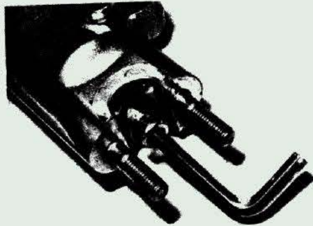
6.2c Remove Allen bolt to release damper assembly
