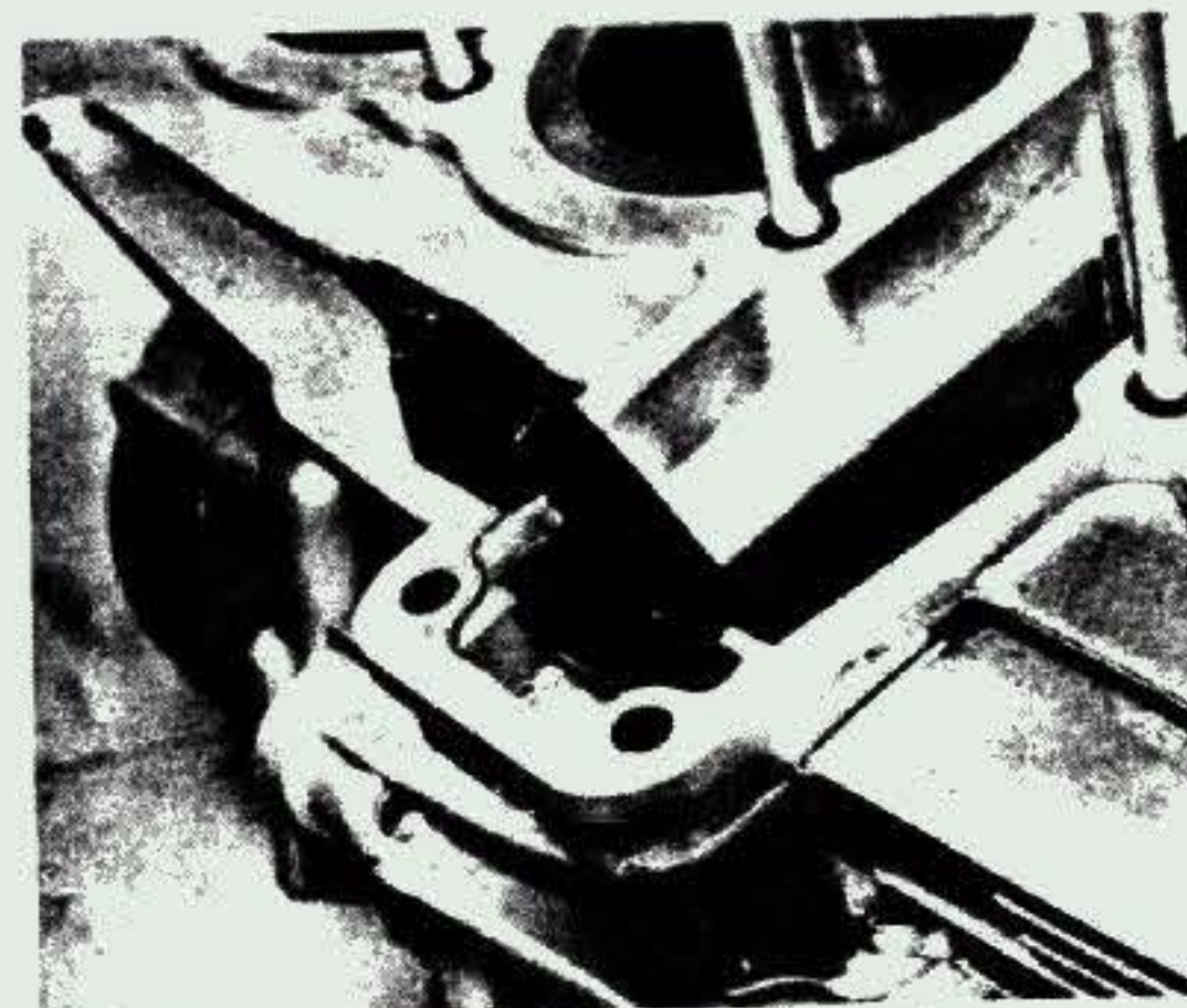
10.2b Chain guide can be lifted away from tunnel
