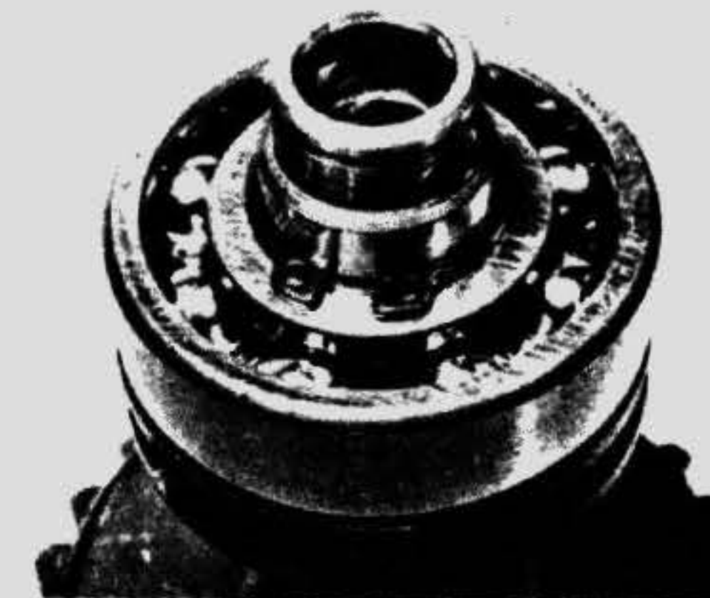
23.2c Bearing retaining circlip can now be released
