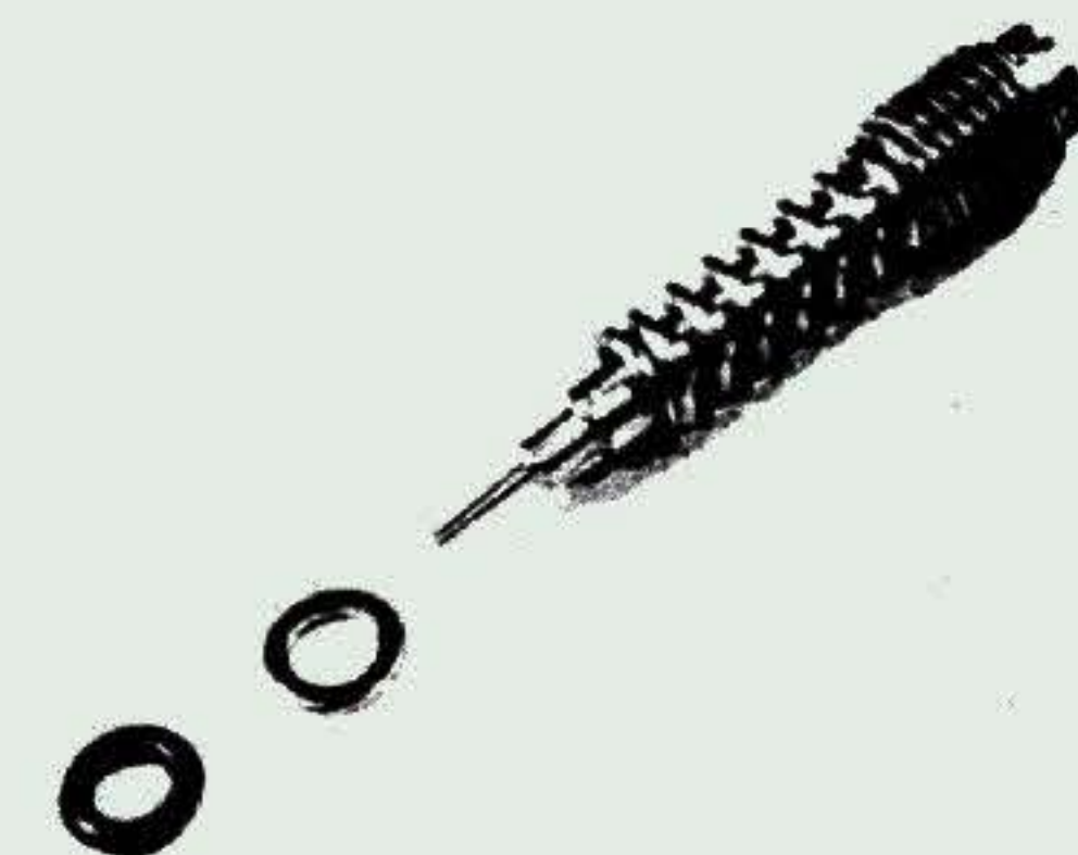
5.11b Pilot screw assembly - note arrangement for washer and O-ring
