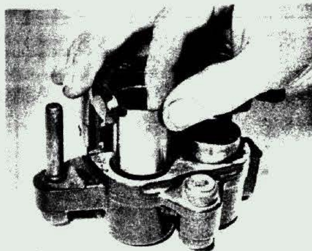
14.2a Remove pistons to check for scoring or corrosion
