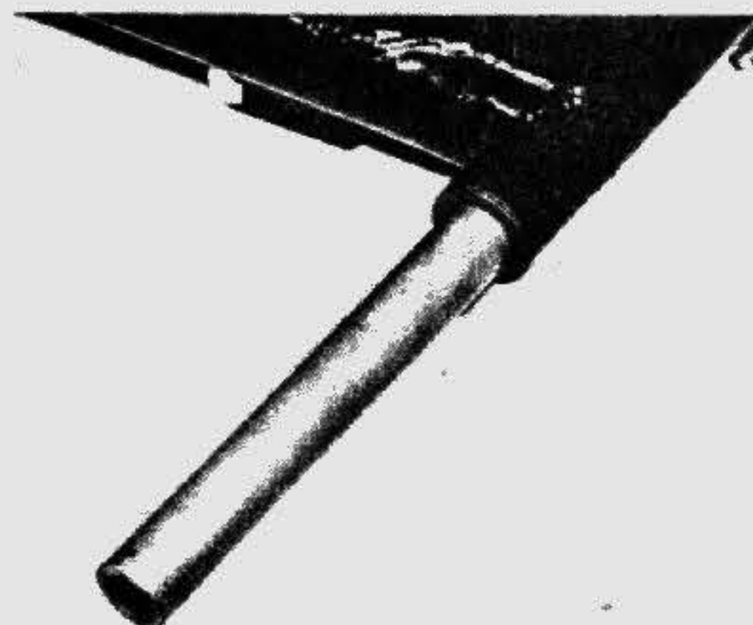
9.6a Remove sleeve and check for wear
