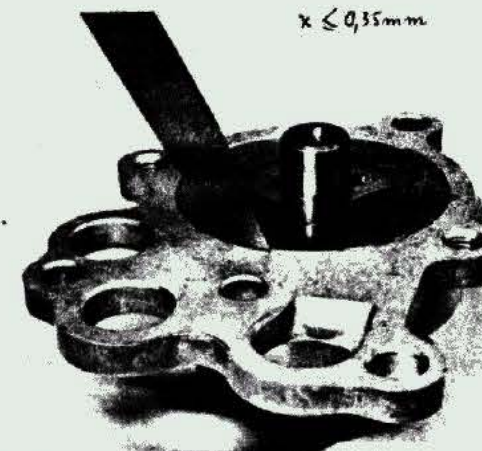
15.5a Measure outer rotor to pump body clearance
