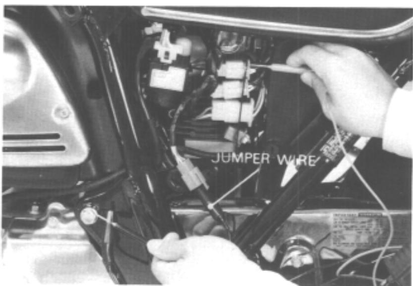
Move the positive voltmeter lead to the yellow wire of coupler B. Voltage should be 12V DC.
